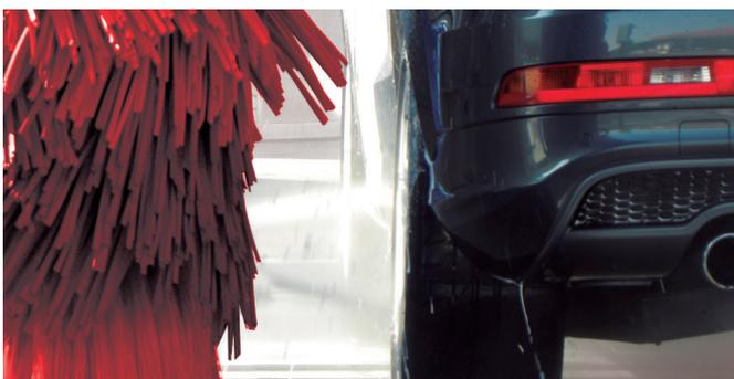
As the ideal complement to high-pressure, we have several wheel-wash systems to ensure thorough rim cleaning: standard or double telescopic disk wheel-wash + high-pressure with 4 or 8 nozzles, or high-pressure wheel-wash with 6 rotating nozzles.
